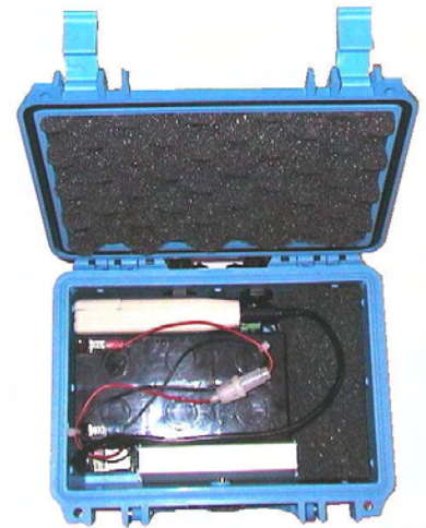
Logger, GSM Modem & Battery in I.P.68 Weatherproof Enclosure
