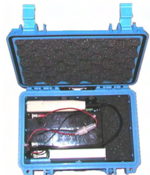
Logger, GSM Modem & Battery in I.P.68 Weatherproof Enclosure
